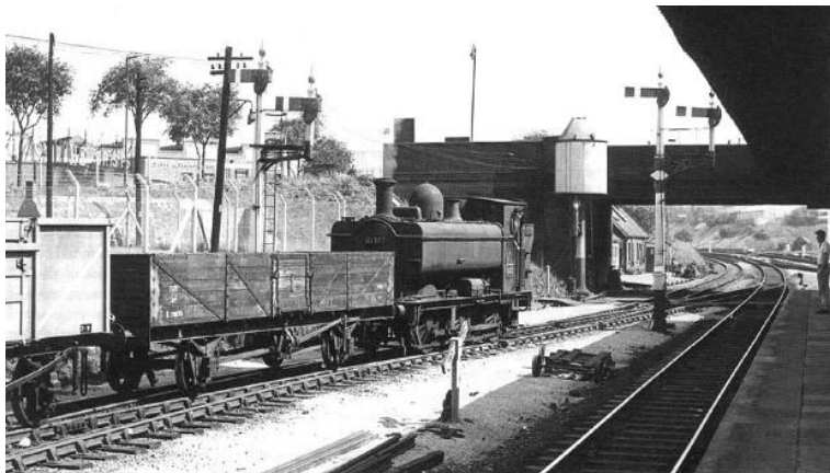
Ex Great Western Railway 0-6-0PT 57xx Class No.8737 shunts a rake of wagons into Tyseley Goods Yard in the summer of 1959. No.8737 was built at Swindon Works in April 1931 and finally withdrawn in December 1962. The water crane by the bridge was surmounted with a conical 3,000 gallon Pillar tank, supplied from the Hockley to Tyseley water main.
