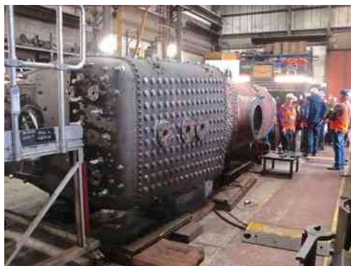
A firebox and boiler on their side in the boiler shop
